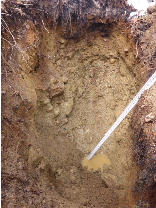
Figure 5- Station 2+50 trench. No bedrock observed, material was primarily sand with gravels, cobbles, and boulders
